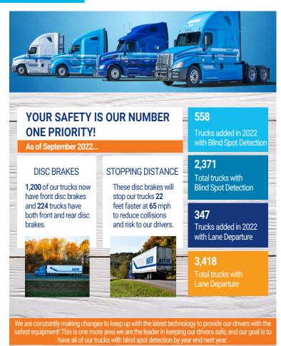
Another safety feature Marten is improving upon is installing disc brakes on all our trucks. Disc brakes allow our trucks to stop 22 feet faster when going 65 mph! Currently, 1,200 trucks have front disc brakes and 224 have both front and rear. These numbers are increasing every month and eventually all Marten trucks will have disc brakes installed.
