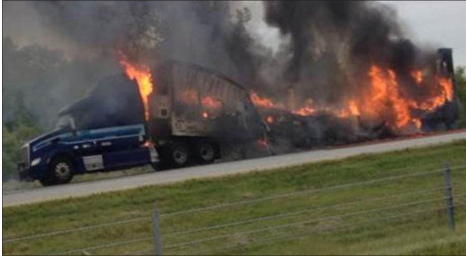
TRAILER FIRES DON'T NEED TO HAPPEN: Research suggests 99% of all trailer fires are preventable! Driver error on a downgrade resulted in this $164,000 loss.
